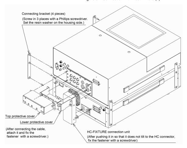
Figure 3.3 Connection with Test Fixture (b)
