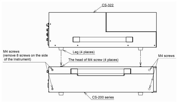
Figure 3.2 Connection with Test Fixture (a)
