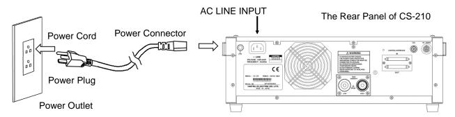
Figure 3.1 Connection of Power Cord (CS-210)
